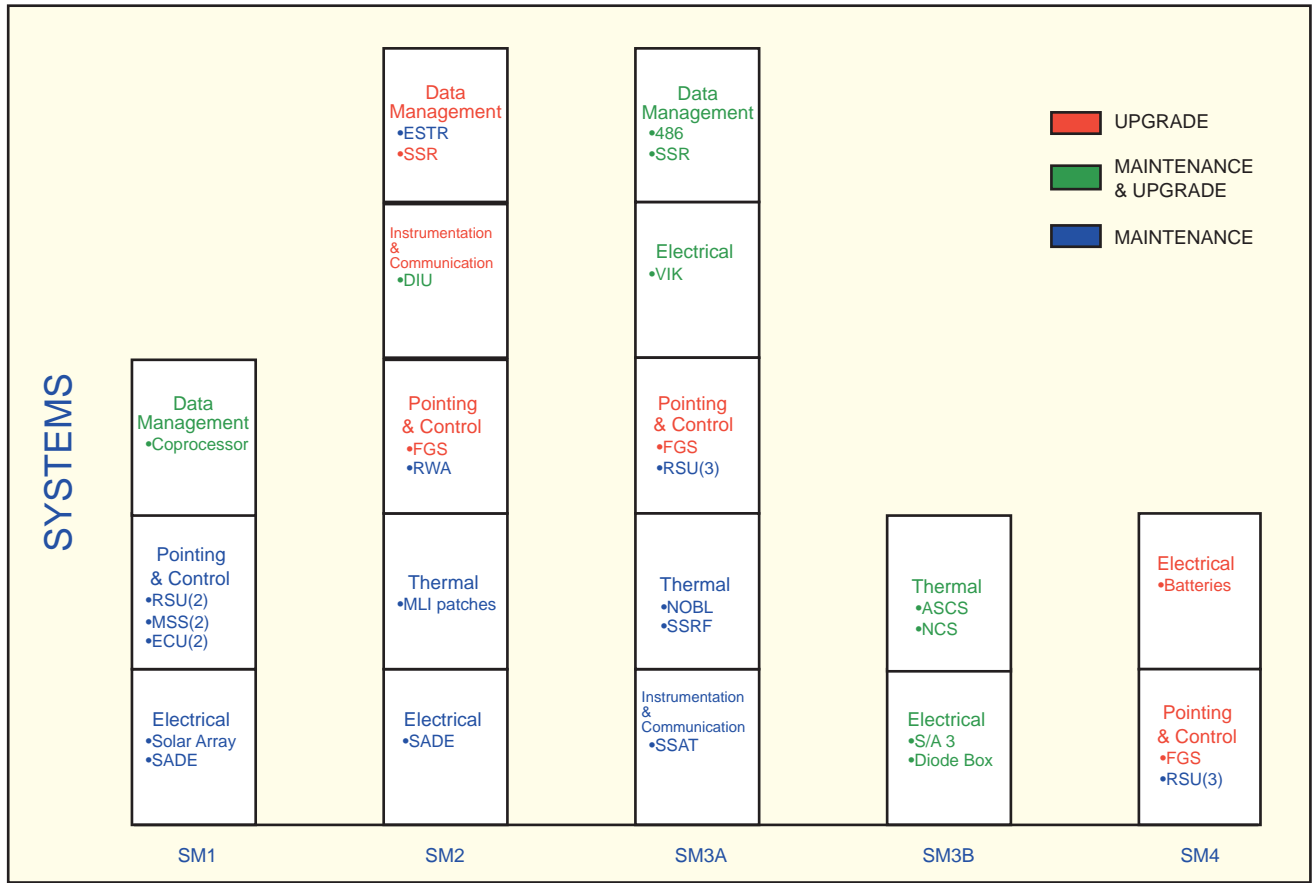
Fig. 7-2 Systems maintained and upgraded during each servicing mission
