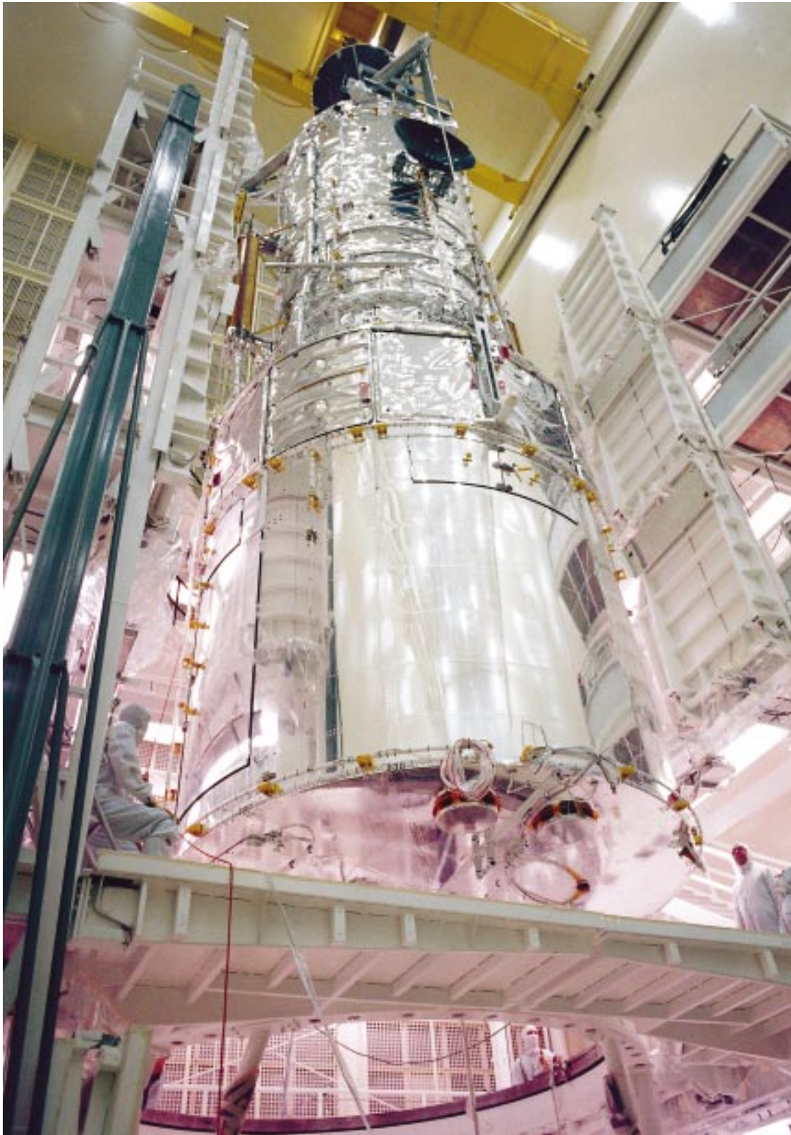
Fig. 1-1 The Hubble Space Telescope (HST) – shown in a clean room at Lockheed Martin Missiles & Space in Sunnyvale, California, before shipment to Kennedy Space Center – is equipped with science instruments and engineering subsystems designed as orbital replacement units.
